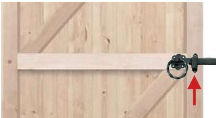
Go to the other side of the gate. Connect ring latch to stainless steel bar, mark holes, remove, drill pilot holes then screw
